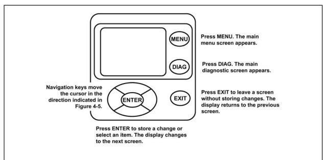
**FIGURE 4-4. Analyzer keypad.** Four navigation keys move the cursor around the screen. The position of the cursor is shown in reverse video. The navigation keys are also used to increase or decrease the value of a numeral. Pressing ENTER selects an item and stores numbers and settings. Pressing EXIT returns to the previous screen without storing changes. Pressing MENU always causes the main menu to appear.
